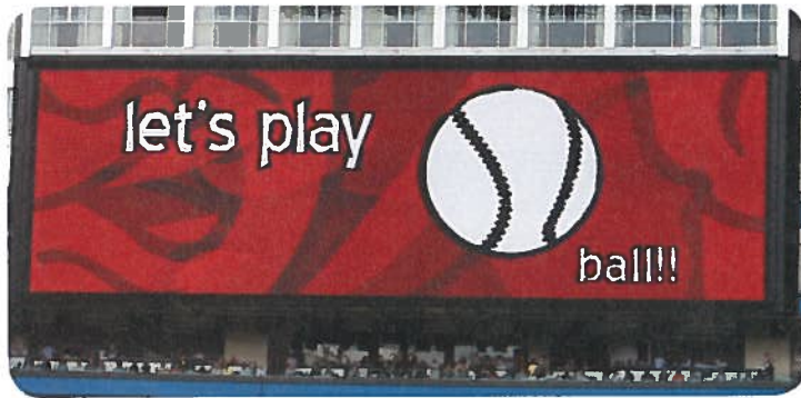
Figure 1 The Videoboard at the Rogers Centre measures 34 m × 10 m and is capable of displaying 4.3 trillion colours.
