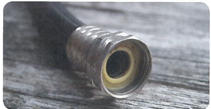
Figure 4 Inside the end of a garden hose is a round washer. This flexible washer works in a similar way to an O-ring.
