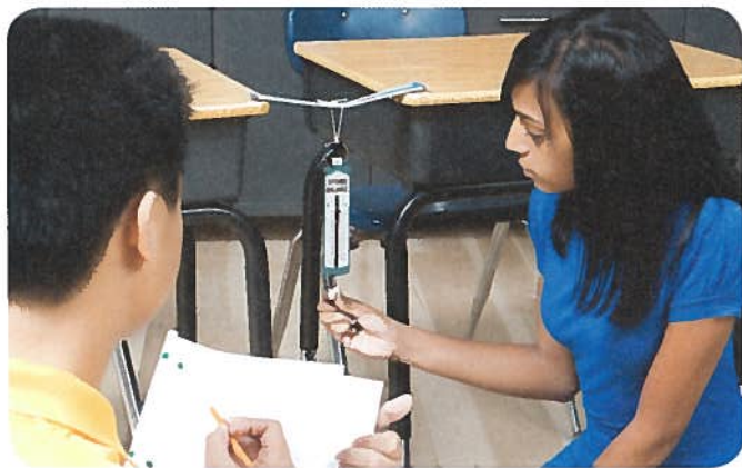
Figure 2 Setup for testing the strength of a beam bridge
