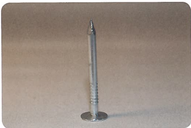
Figure 6 A roofing nail is rustproof and has a large head and a notched shank to hold down the shingles in windy conditions.
