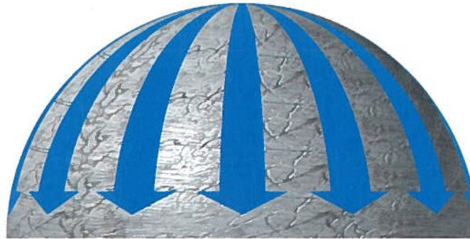
Figure 9 The compression force on this dome is directed downward in many planes at once.
