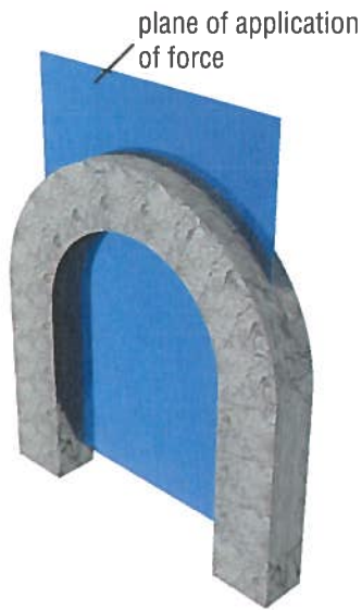
Figure 8 The compression force on this arch is directed downward in a single plane.
