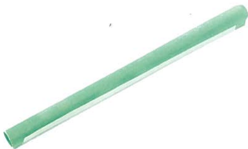
Figure 1 A building rod constructed out of scrap paper
