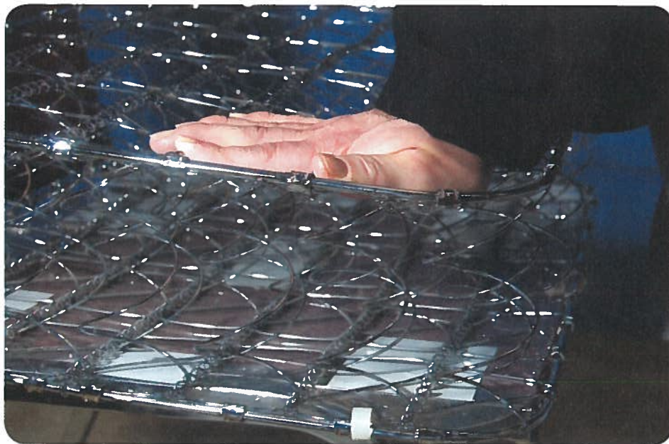
Figure 5 These mattress springs have compression forces acting on them.
