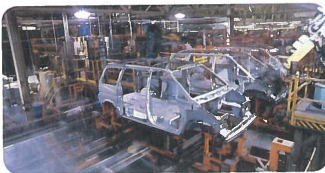
Figure 7 This automobile chassis is a combination structure with both shell and frame components.
