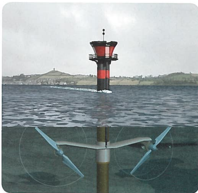
Figure 3 Underwater turbines may capture both tidal and flowing river energy and convert it into electricity.
