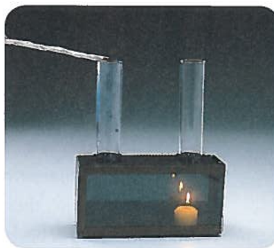
Figure 3 The burning candle is placed beneath one chimney; the smoking paper is held above the other one.
