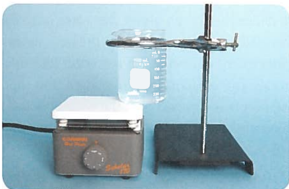
Figure 2 Setup of the beaker on the hot plate
