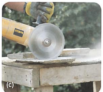
Figure 7 (a) A rough diamond found in a mine, (b) a cut and polished diamond set in a ring, and (c) an industrial diamond in a saw blade
