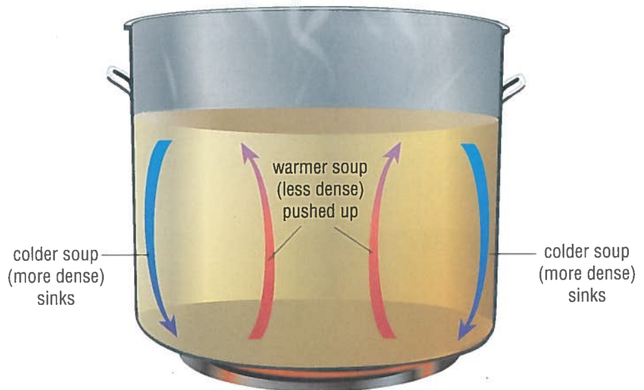
Figure 1 Soup is heated by convection.
