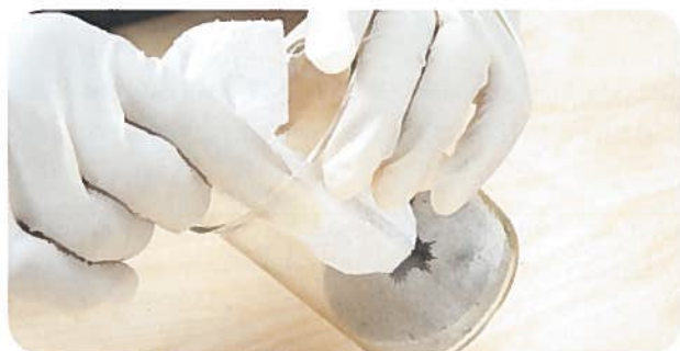
Figure 2 Separating the parts of mixture #2 by magnetism
