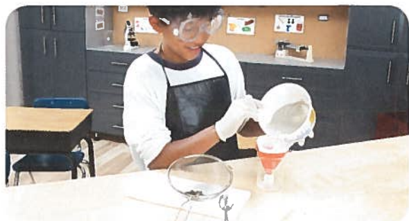
Figure 3 Separating the parts of mixture #3 by filtering
