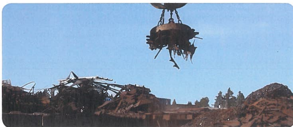
Figure 5 This magnet separates scrap metal so that it can be recycled and reused.
