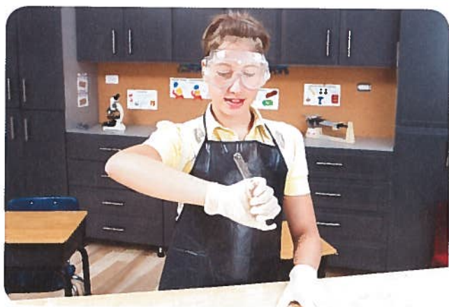
Figure 1 To mix samples in a test tube, fill the tube no more than halfway. Put a stopper in the test tube, and put your thumb firmly over the stopper. Holding the test tube away from you, gently turn it upside down two or three times. Wear gloves when mixing samples this way.
