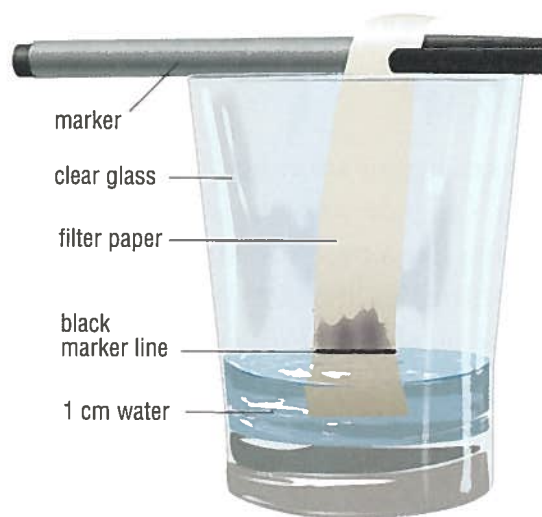
Figure 4 Use the clip on the marker lid to hold the paper away from the side of the glass.
